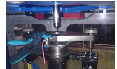
Fig. 1: Experimental set-up for droop test impact on composite
