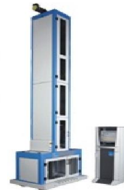
Fig. 1: Experimental set-up for droop test impact on composite
